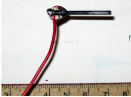
Place a glob of hot glue around the wrapped graphite rods.
