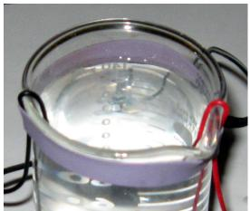
Place a rubber band around the beaker to hold the wires firmly.
