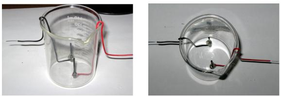
Place the wires into a beaker and bend into place as shown.
