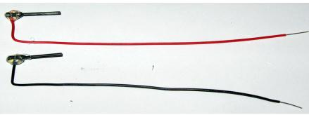
Bend the wires in a 90deg angle as shown.
