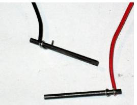
Carefully wrap the wires around the graphite pieces.
